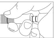
• Never use the airmotor, if the attachment cannot be smoothly installed onto or removed from the airmotor. In this, consult the Patterson Service Center.
